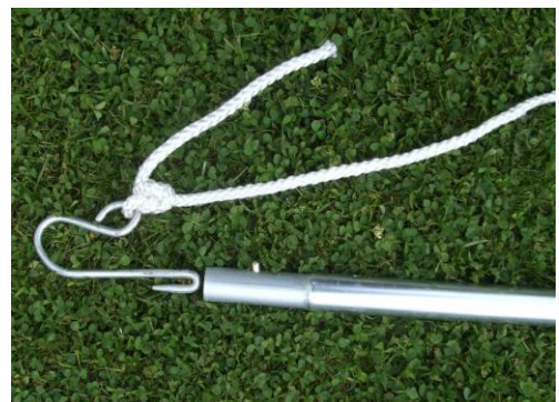
Figure 11; Ridge pole, frame and side ropes (left) and side ropes tied to hooks (right).
