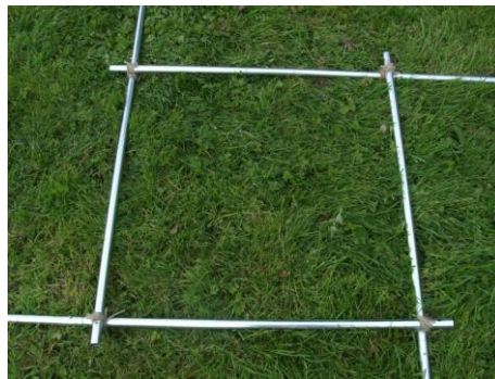
Figure 10; Layout and cross lashing of joints.
