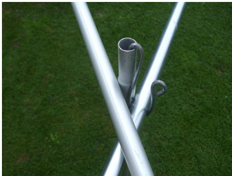
Figure 12; Hook in the open end of the supporting rod (left) and fully elevated frame (right).
